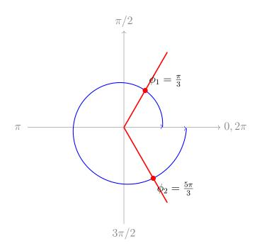
The diagram shows the two solutions for  $\phi$  in the interval  $(0, 2\pi)$ .
